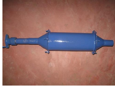
Fig 8: SCR pipe of this project
