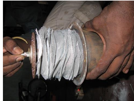
Fig 8: Inner body placed inside of outer body
