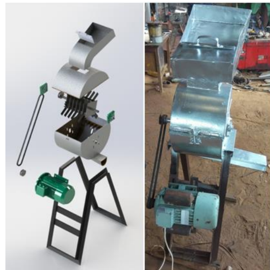
Fig. 3 Optimized CAD Model and Constructed Fibre Milling Machine
