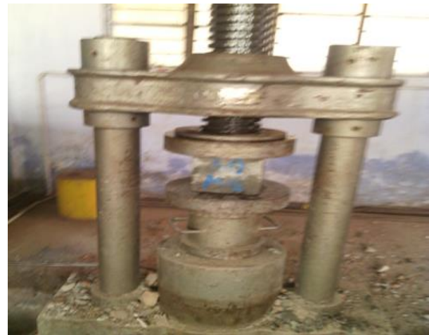
Figure 2 Compressive strength test
