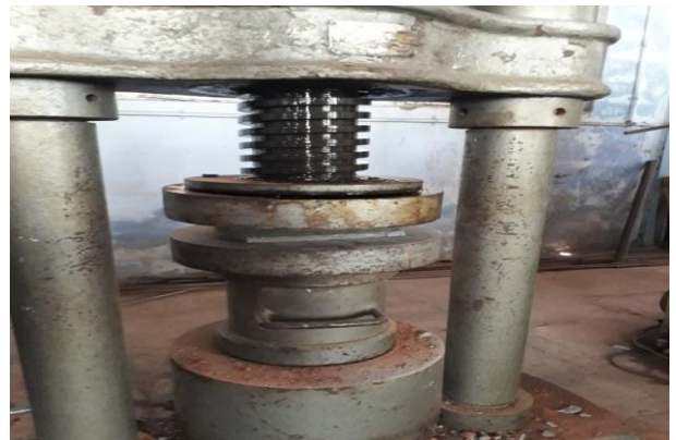
Fig 4.1: Compressive testing of specimen
