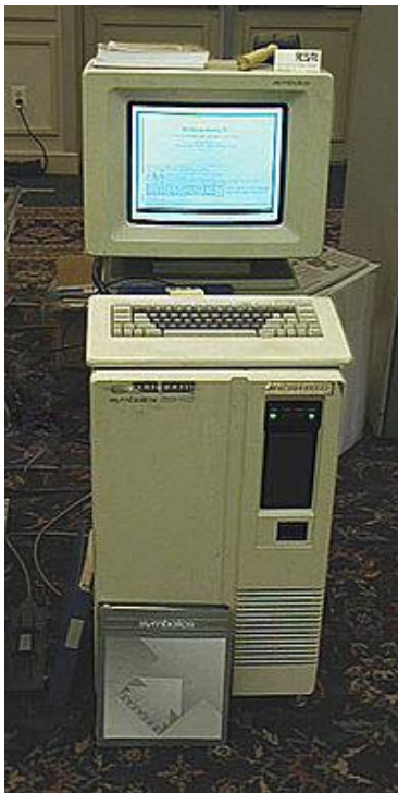
Fig. 2: A Symbolics Lisp Machine: an early platform for expert systems
