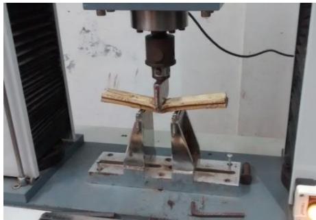
Fig. 3 Three point bend test of four layered laminate
