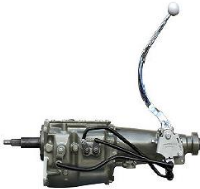
Fig.1 Manual Transmission Gearbox [2]
