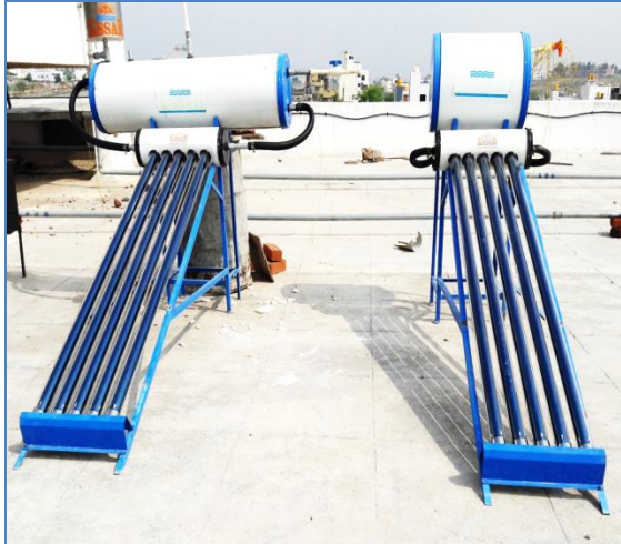
Fig. 7 Experimental set up of EVTC with both conventional and Normal tank
