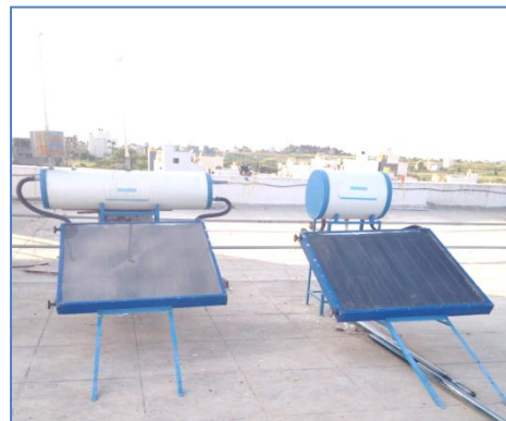
Fig. 6 Experimental setup of Heat Exchanger tank with EVTC
