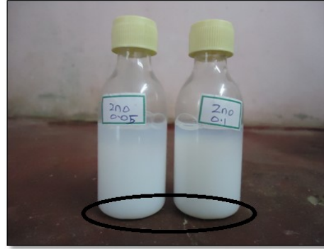
Fig. 8: ZnO After three days (Zno (0.05%) Zno (0.1%))
