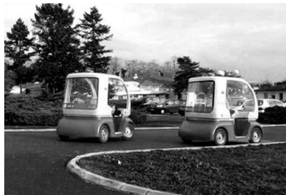
Fig 2 . The driverless vehicle (left) passes the halted vehicle (right) (drive on the right).
