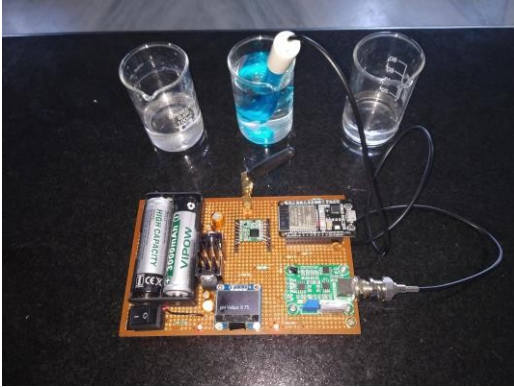
Fig.3. Experimental setup of Sensor node
