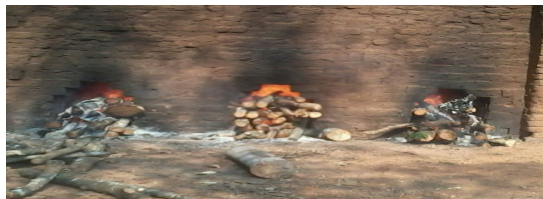
Fig. 7 Initiation of fire by feeding firewood through air holes at the bottom
