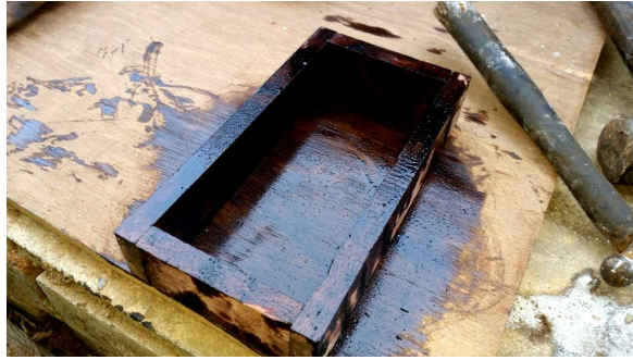
Fig 1. Brick mould of size 190 x 90 x 40mm
