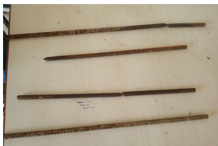
Fig 3(a) Failure of newly manufactured steel bars
