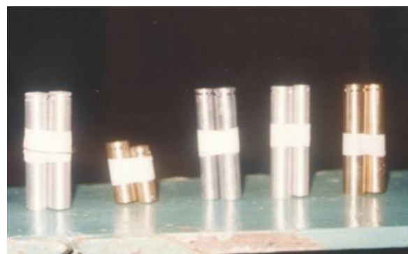
Fig. 1: Casted and Machined Anodes Produced Locally
