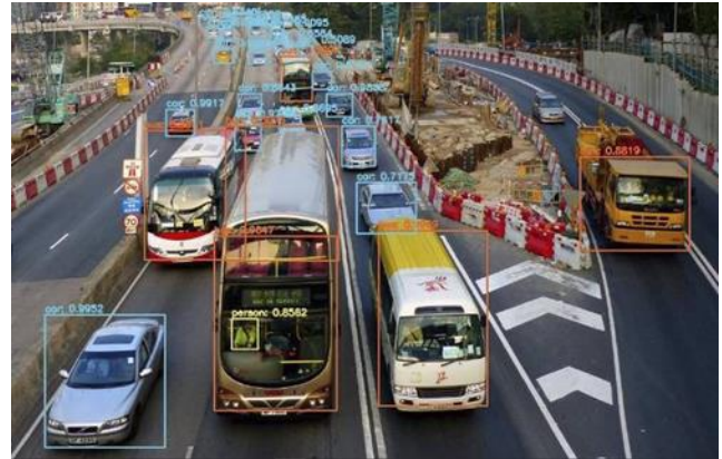
Fig -6: Detecting vehicles in traffic
