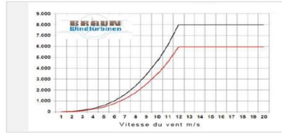
Fig. 5.0: Power curve of 2.5KW ANTARIS Wind Turbine.
