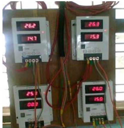
Fig.4. Charging Voltage and Current of Each Controller
