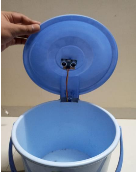
Fig.5. HC-SR04 Ultrasonic Sensor attached to dustbin
