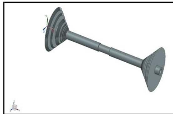
Fig.5: 3D modeling of one-piece drive shaft
