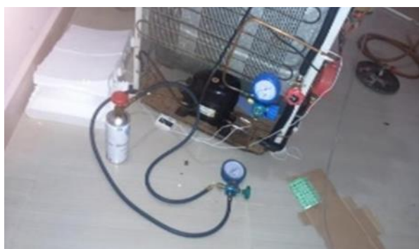
Figure: Gas Charging
