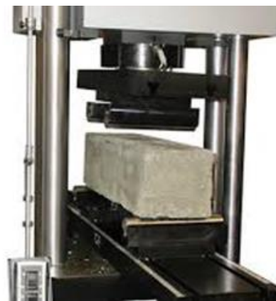
Figure 3: Flexural strength test
