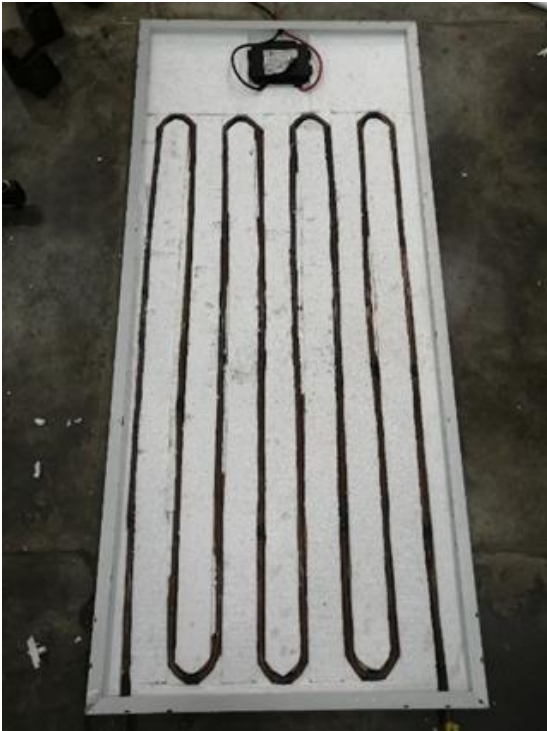
Figure.2 Cooling system of solar photovoltaic thermal collector
