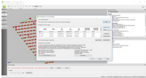
Fig.4: Importing the measured or acquired GCPs/Checkpoints
