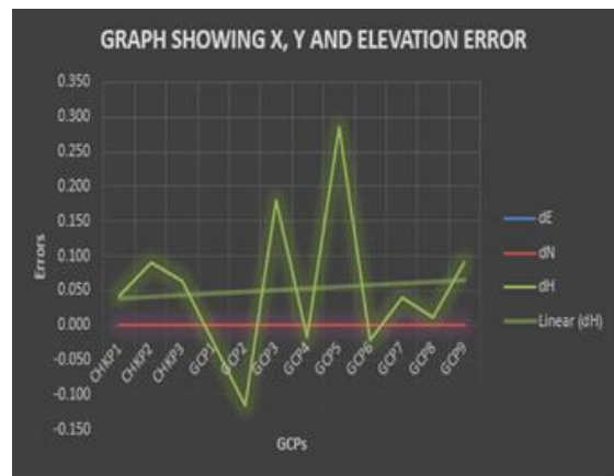
Fig.11: Easting, Northing and Elevation Errors using a graph
