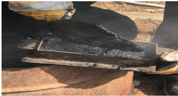
Fig 2.6: Transfer of LDPE, PET and Sand Blend into the mould
