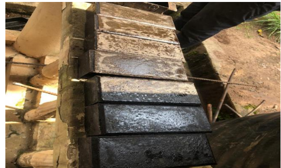
Fig: 2.11: the control samples of the interlock tiles after drying
