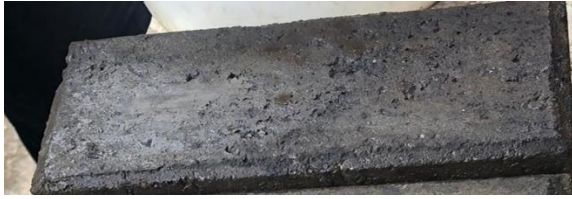
Fig 3.1 Porous Surface of the PET: Sand Blend
