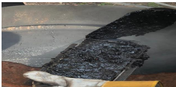
Figure 2.5: Transfer of PET: Sand Blend into the mould
