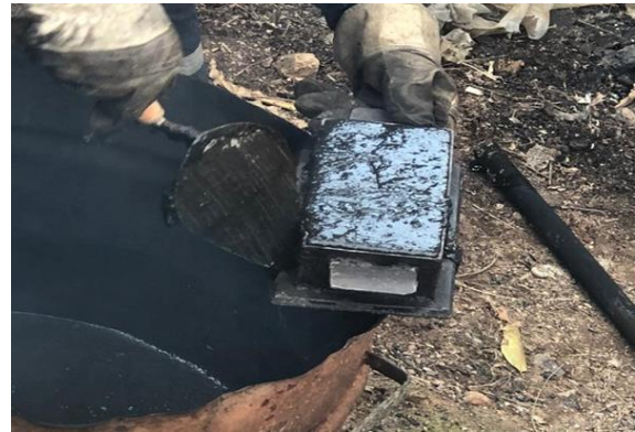
Fig2.3: Transfer of LDPE: Sand Blend into the mould
