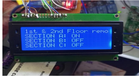
Figure 10a: Section B & C of the Senate Building turned OFF to meet the load requirement
