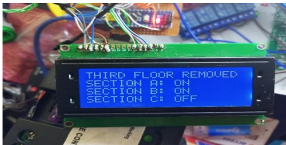
Figure 9a: During peak hour Section C turned OFF
