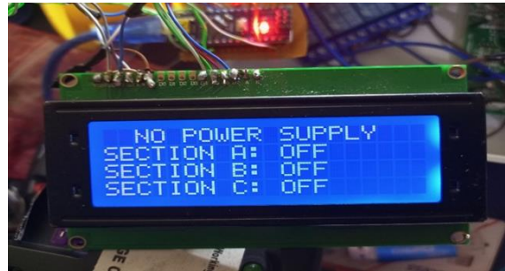
Figure 7a: Initial State when all load is off
