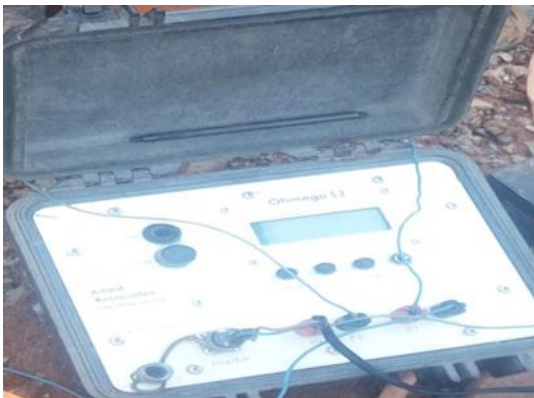
Figure 4: Picture of an Omega resistivity meter showing its interface.
