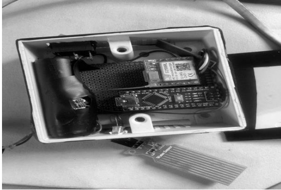
Plate 3: Circuit design on Veroboard
