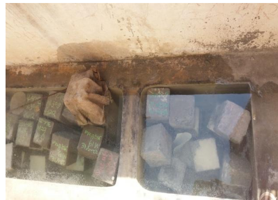
Fig No.6 Curing Of Cubes in Curing Tank
